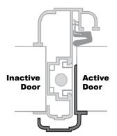
Add the Astragal Security Strip to any outswing double door combination for added security and clean finished appearance eliminating the reveal between the doors
